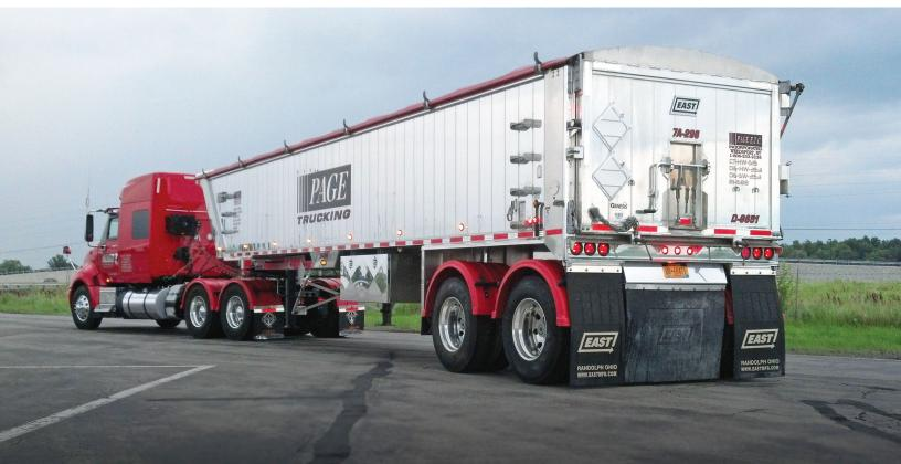
with 5 foot-tall side walls, uses high-quality aluminum, which improves resale value and keeps Page Trucking's trailers looking good. Because Page Trucking owner operators take pride in their equipment's appearance, they like the smooth-sided Genesis<sup>®</sup> side walls that are easier to clean and do not show dents from the inside. And, the trailers have superior dump stability, giving drivers more confidence.
