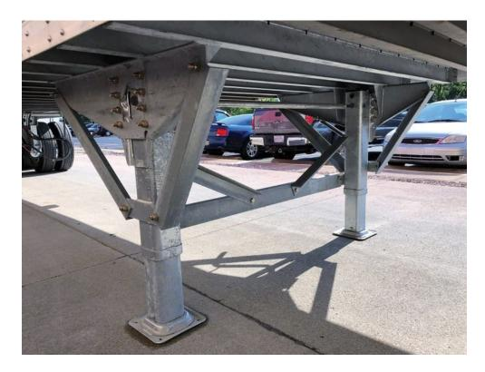
Corrosion-prevention options, such as galvanized landing gear, are a smart option for trailers operating in harsh winter conditions.
