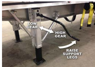
Figure 6: Landing Gear Operation
