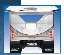
At East, we put ourselves in the driver's seat when we design trailers. Maybe that's why we never liked the half-round trailer design – because we wouldn't feel comfortable pulling one. Compared to our square-box trailers, they lack the inherent rigidity to resist twisting, and that makes them less stable when dumping. And they have a much higher center of gravity, making them harder to corner and more prone to turn over.
